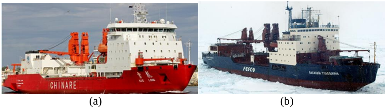
Fig. 1.21. Multifunctional Chinese ship for Arctic «Xue Long» (a), originally is built by the design # 10620 at the shipyard of KSPA and reconstructed at the shipyard in China, the ship «Vasily Golovnin» of the same original design (b)
