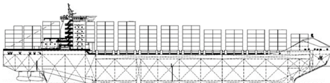
Fig. 1.33. Ice-class container ship of Arc7 category conceptual design of 3000 TEU capacity ( www.morvesti.ru )
