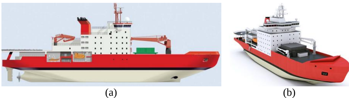
Fig. 1.12. Multifunctional ice–navigating ship for the Government of Argentine ( http://akerArctic.fi/ )
