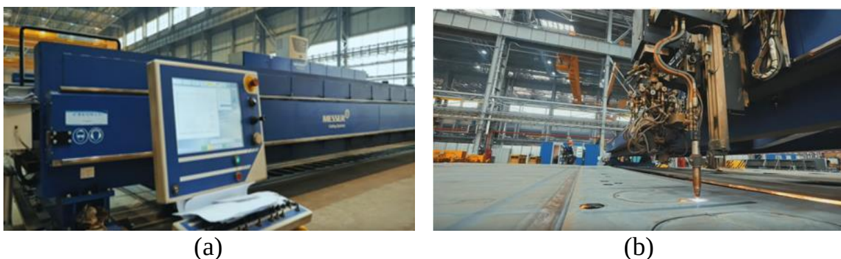
Fig. 9.5. Installation for automated plasma cutting of steel sheets up to 300 mm thick for construction of ships' hulls parts
