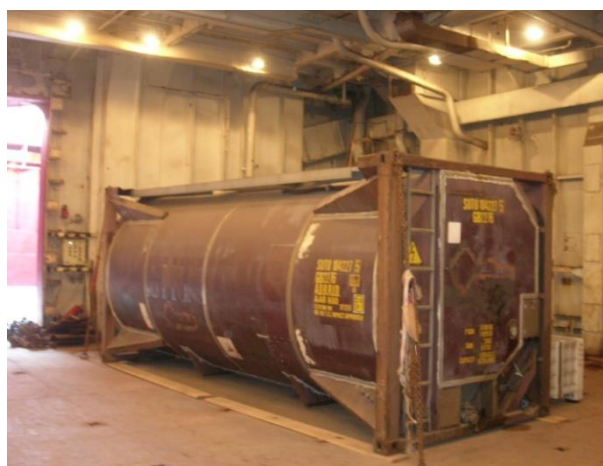
Fig. 4.9. Tank-container for liquid cargo in the hold of icebreaking-supply ship of the design #10620
