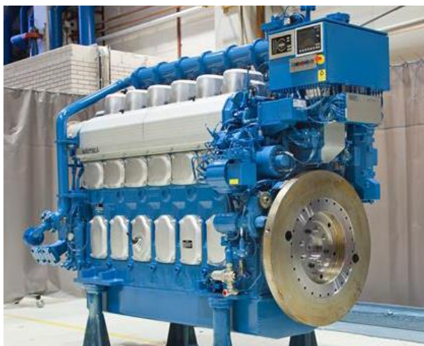
Fig. 4.6. Gas–diesel engine Wärtsilä 20DF for ship ( www.wartsila.com )
