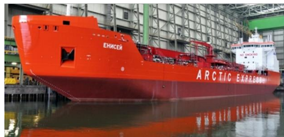
Fig. 1.32. Arctic tanker for transportation of oil products «Yenisei» ( http://izvestia.ru/ )
