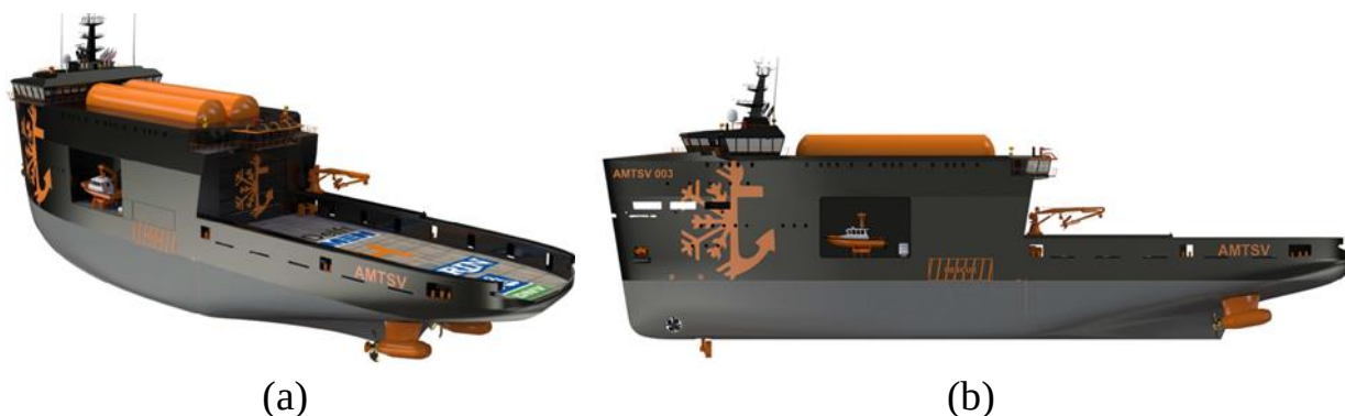
Fig. 1.19. Design of the arctic modular towing supply ship for the service of offshore platforms, cargoes and supply delivery and for towing ( www.damengears.com )
